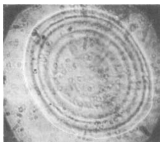
Fig.10. Microphotographs of free cholesteric drop obtained with a specimen having 2% of CEC. a) Using plane polarized white light. Crossed polars 120x. b) Using sodium yellow light. Crossed polars 110x.
